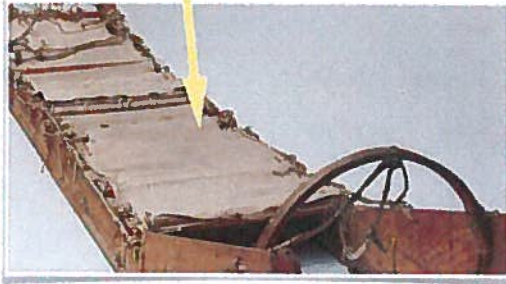
Example of a sled with skins tacked down over the seat frame
