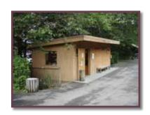
STORAGE SHED: A small, 120-square-foot storage shed located behind the ranger station is used for storage of gasoline, gas powered tools, and other flammable maintenance implements. The shed is in poor condition, does not adequately meet storage needs. Tools and other supplies for other Ketchikan area parks are stored in it further reducing available storage space. It is in plain view of visitors from the parking area and detracts from the visitor experience.
